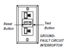
button should pop out, shutting off the circuit. If it doesn't, the breaker is not working properly. If you don't test them once a month, the breakers have a tendency to stick and may not protect you when eeded.
